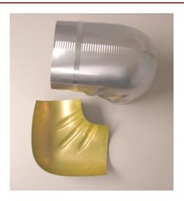
ITW Multi-Fit Aluminum Elbow Covers are designed to yield a 5/8" overlap at the heel and throat joints when used over insulation that complies with the target diameters in ASTM C585 and C450. If the insulation outer diameter deviates significantly from that specified in these standards, the overlap size may change and the fit may be compromised.
