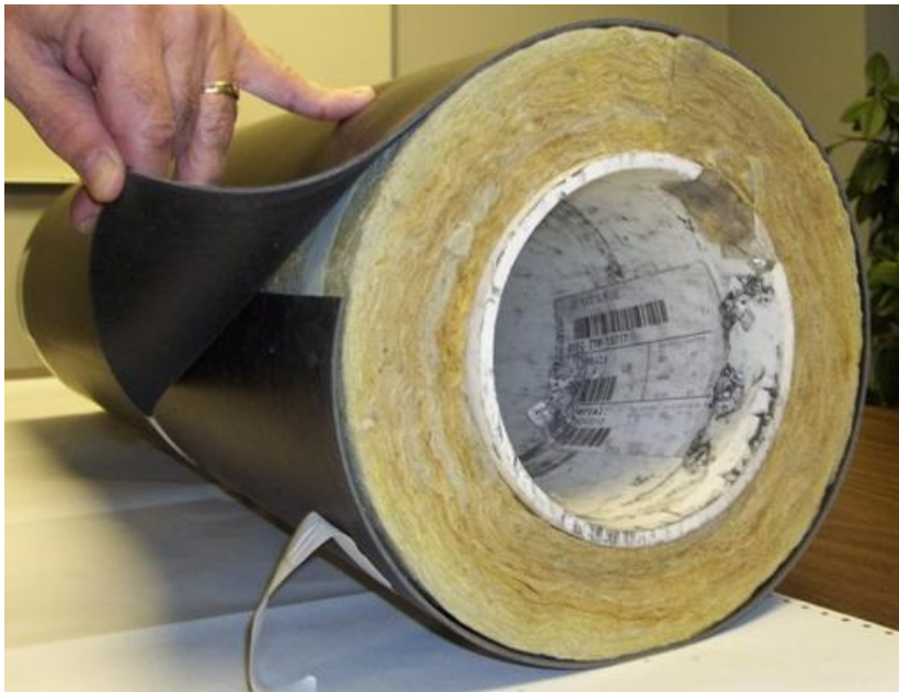
Figure 3 – Mass loaded vinyl with required \geq 5.1 cm (2 inch) longitudinal overlap. Joint located at about 3 o'clock position.
