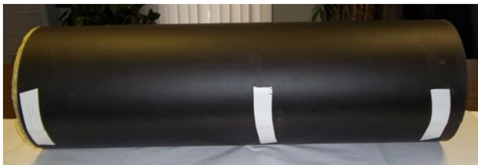
Figure 4 – Mass loaded vinyl secured lightly with tape.
